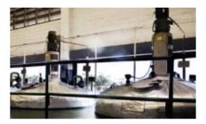
Our main blending platform consists of 8 vessels ranging in capacity for 4,000 litres to 45,000 litres. These vessels blend both automotive and industrial oils and are dedicated to product families to eliminate cross contamination issues. Smaller vessels are available for low volume or specialty products.
